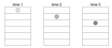
Signal strength of the circular defect increases as it passes through each stage
