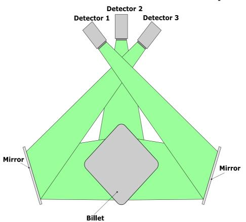
There is no imaging required since the photo detection is only interested in the return fluorescence and the fact that the laser beam is an almost parallel light beam. The only light received is that from the MPI indication, illuminated by the laser spot.
