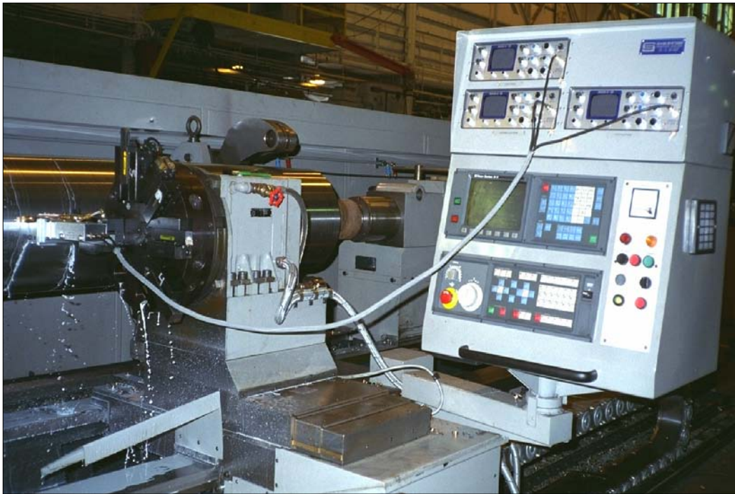
Figure 4 - The Ultrasonic System Inspecting a Roll
