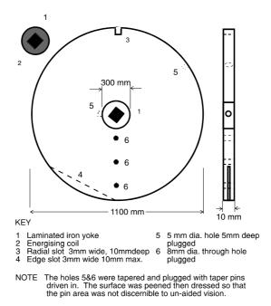
The limitation of the induced current method is only the size of the central hole relative to the outside diameter of the component. It will be understood that even with laminations there is a saturation value which depends on the cross section area of the yoke. By experience this limitation can be expressed by the cross of yoke is greater than and equal to the square root of outside diameter of the part to provide a field of 5kA/m.
