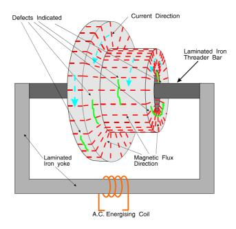
For parts with holes a more efficient method is the induced current method in which current is induced to run round the circular part by a laminated yoke threader bar system energised by an AC coil around one limb of the yoke. As illustrated above.
