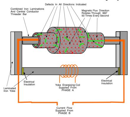
In schematic terms a magnetising arrangement is shown. The threader bar is a composite of iron lamination and copper conductor as shown. Since the laminations are conductors it is important that there is insulation between the copper conductor and the lamination. Further to prevent recirculation currents there is insulation between the limbs.
