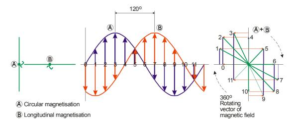
Applied to the magnetising of hollow parts this means that the induced current is derived from one phase of a three phase mains supply and the central conductor current from a different phase. As there is a phase lag the resultant vector of the two simultaneously induced fields changes its angle in direct relation with the magnitude of the flux in each of the primary directions. Therefore with a phase difference of 120° the field will rotate through 360° at mains supply frequency.
