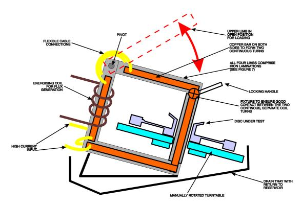
The photograph is of a typical machine for testing railway brake discs. These applications are manual but there is no reason why the system should not be applied to automatic systems.
