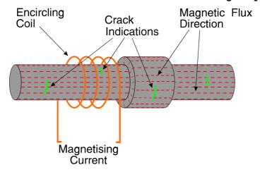
E1444 has coil incremental formulae for testing purely cylindrical parts but, for very good reasons does not address parts with varying cross section. An encircling coil will not induce a field in the required direction to reveal circumferential flaws on the end face or sections of the part not longitudinal.
