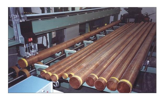
This equipment is to provide both ultrasonic and eddy current inspection of tube and bar products. The ultrasonic inspection is achieved using a number of adjustable Water Column Coupled Probe (WCCP) units for shear wave longitudinal flaw detection and fixed WCCP unit for thickness monitoring. The eddy current inspection uses differential probes mounted in holder attached to the **WCCP** units. See the reverse of this brochure.
