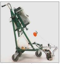
These trollies pushed are steel over plate ensuring the surface completely covered, while, the ultrasonic system monitors the signal from the transducers in
