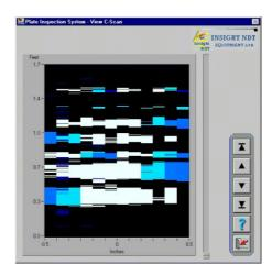
A typical C-Scan from the plate testing software is shown above.
