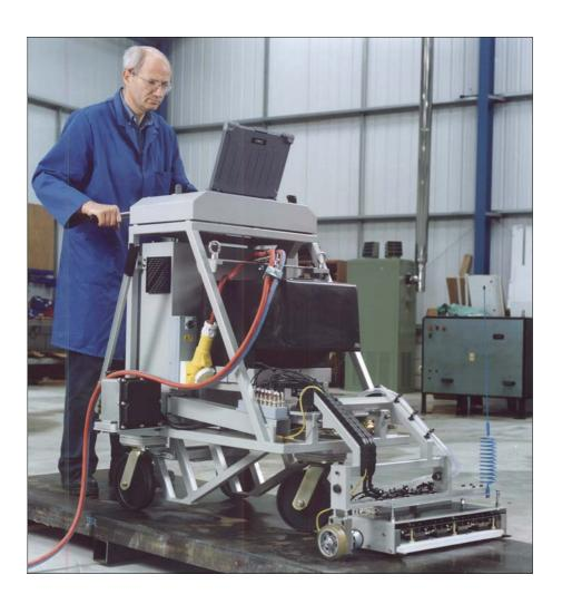
This equipment is a convenient and easily mobile trolley which is manouvered around the plate to ultrasonically inspect plate products. See the reverse of this brochure.
