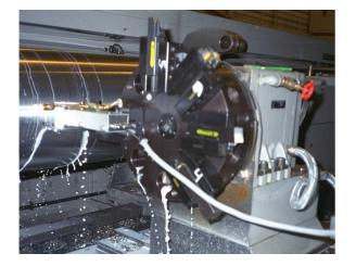
The CNC lathe operator initiates the test by entering the roll diameter and the barrel length into the system. This information will be used by the system to generate a CNC program which would position the ultrasonic probe assembly to maintain the 0.3mm gap and automatically select an appropriate roll RPM to ensure that the peripheral speed of the roll would be approximately 600mm/s.
