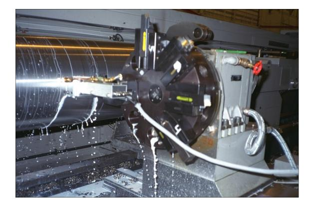
This equipment is for the ultrasonic inspection caster rolls following a period of service but prior to machining them in a CNC lathe. The ultrasonic inspection is carried out using a single fixed **W**ater **C**olumn **C**oupled **P**robe (**WCCP**) unit for the longitudinal shear wave flaw detection in both directions. See the reverse of this brochure.
