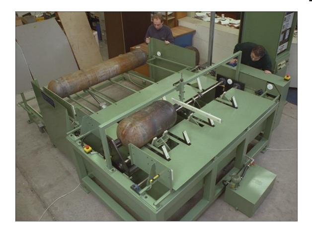
This equipment is for the ultrasonic inspection of seamless gas cylinders. The ultrasonic inspection is achieved using a single fixed **W**ater **C**olumn **C**oupled **P**robe (**WCCP**) unit for both the longitudinal and circumferential shear wave flaw detection in addition to the compression wave thickness monitoring. See the reverse of this brochure.
