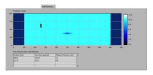
The flaws are represented graphically on the chart. In addition to this chart, there is a single text control which displays the area, position and minimum thickness of the wall thickness flaws found.
