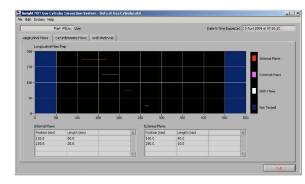
This gas cylinder software has been specifically designed for Ultrasonic Inspection of seamless gas cylinders to BS5045, EN1964 and ISO11439 on a 100% inspection basis.
