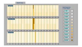
Each line in the C-Scan image is a different channel; therefore in the above case there are 3 channels assigned to the Top bond inspection, 2 channels for the Bottom bond inspection and a single channel for the Back bond inspection.
