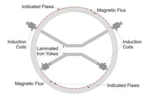
The third yoke magnetises a short length of the bevel of the pipe, by generating an A.C. flux between the pole piece ends across the end thickness. The three yokes will reveal all longitudinal and radial flaws.
