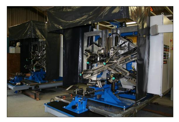
This equipment is specifically for use in detecting surface and near surface discontinuities at the ends of S.A.W. pipe regardless of direction. The system will inspect both ends of the pipe simultaneously up to 500mm in from each end.
