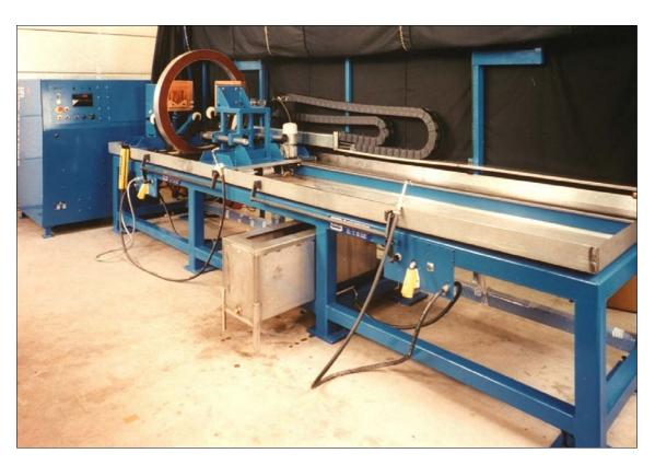
This equipment is for the magnetic particle inspection of large aerospace components such as engine shafts. The machine provides motion control of the coil and the tailstock, thus ensuring a quick and easy set-up from component to component. These features are programmable, thus further reducing the change over time for any given component. See the reverse of this brochure.
