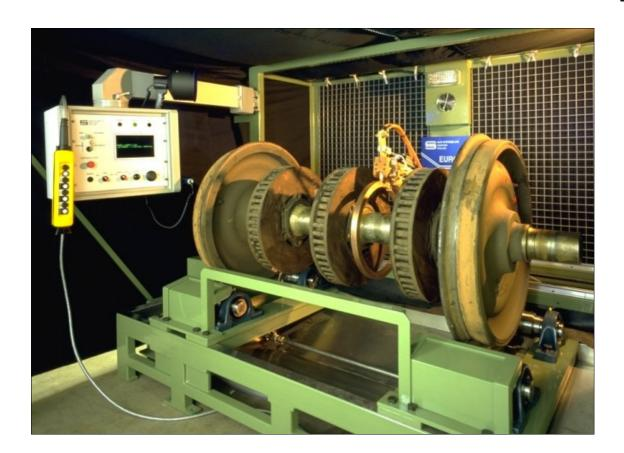
Railway axles which have been in service are routinely tested for surface breaking cracks. One method of testing is the highly sensitive Magnetic Particle Inspection technique which detects any fatigue cracks on the axle. See the reverse of this brochure.
