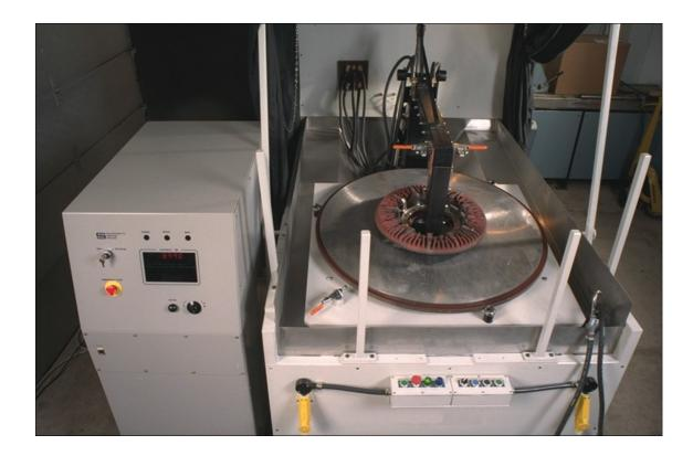
This equipment is for the magnetic particle inspection of disc shaped components in a single non-contact magnetizing shot. This is achieved using a threader bar which is a composite of iron laminations and a copper conductor. Therefore it is necessary that the disc have a central hole large enough for the threader bar to pass through. See the reverse of this brochure.
