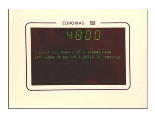
Control of the power pack is through the screen dialogue and simple rotary control and "ENTER" button. The active unit settings are displayed on the screen which also incorporates a large digital ammeter with reading hold facility.
